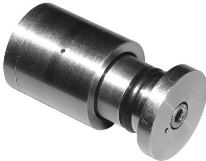
Figure 5 O-ring RGD test fixture comprising spigot, body, and end caps
