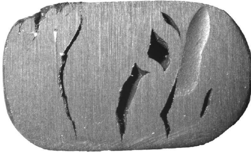
Figure 11 HNBR4 section after Test 3, standard groove
