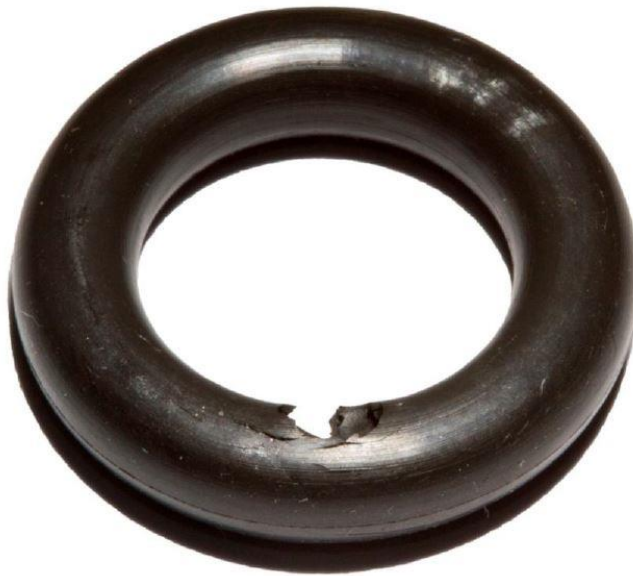
Figure 3 Fluoro3 seal after CO 2 RGD test, showing material loss due to local extrusion
